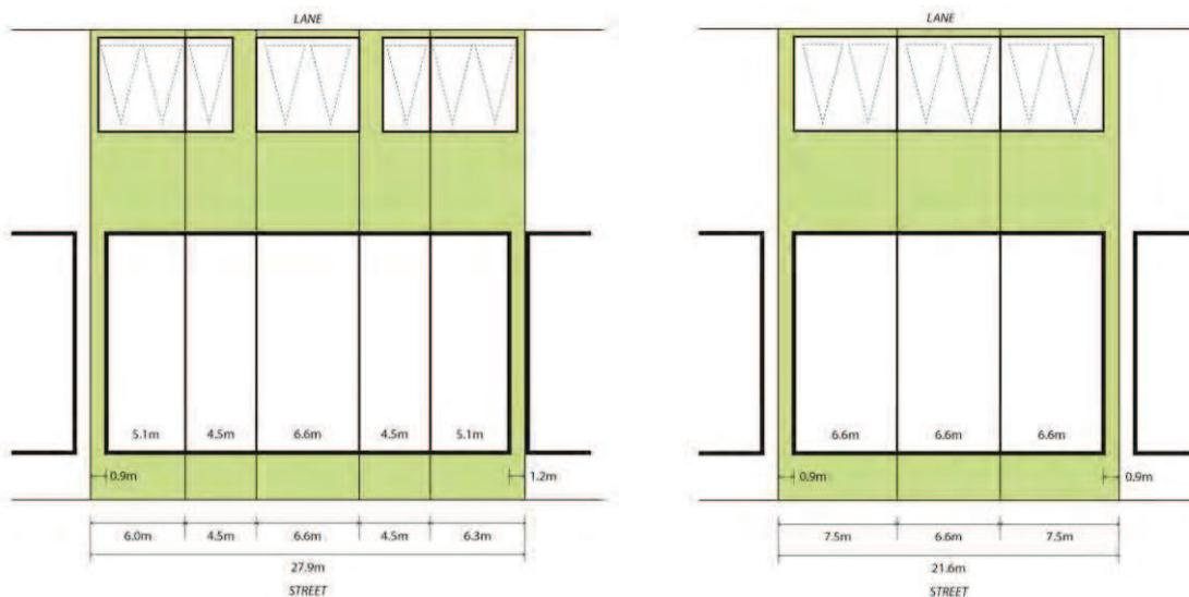
**Figure 8** Two examples of lot subdivision for 'sets' of attached or abutting terraces.
